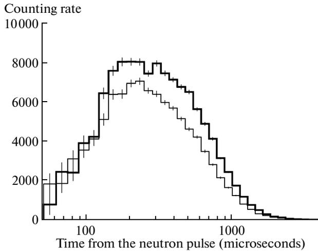
**Fig. 1.** Examples of DAN measurements for time profiles of thermal neutrons (energies  $<0.4$  eV) along the time scale with zero moment corresponding to the initial pulse of 14.1 MeV neutrons from the PNG. The numerical simulations show that two measured time profiles shown by bold and thin lines correspond to maximal 3% and minimal 1% estimations of water content, respectively.
