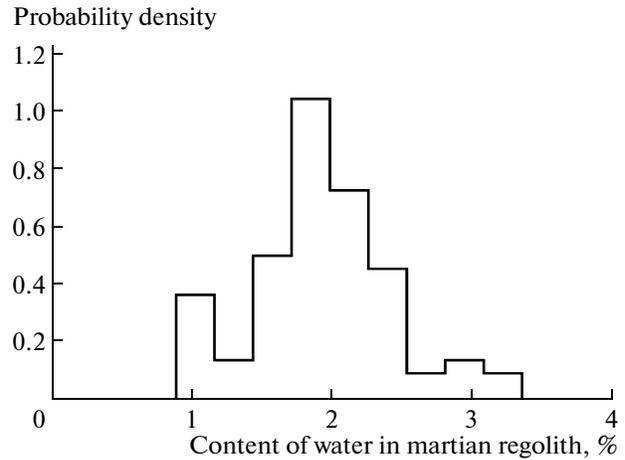
**Fig. 2.** Distribution of the average content of water in the upper most layer of 60 cm along the rover traverse for the 1st year of DAN operations.
