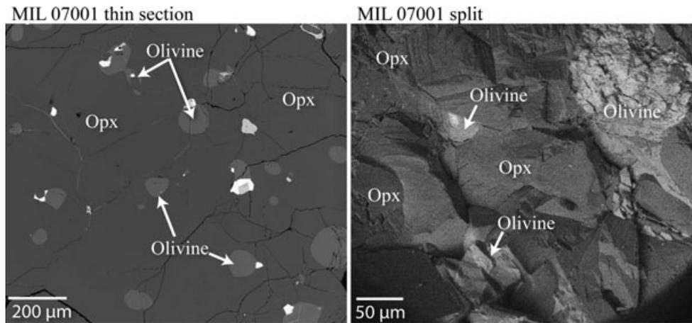
Fig. 2. BSE images from the MIL 07001,2 thin section (left) and the MIL 07001 coarsely ground sample split prior to powdering for spectral analysis (right). The thin section and split show similar phase abundances and textures. Note the images were taken at different magnification levels and at different analytic conditions; the latter leading to phases having different grayscale thresholds between images.
