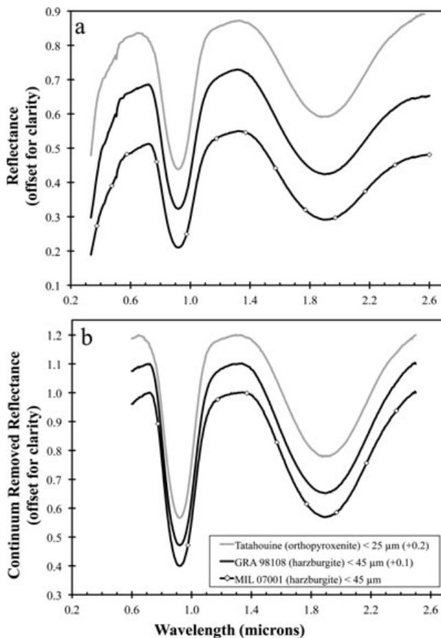
Fig. 3. a) VNIR reflectance spectra of harzburgitic diogenites (ol + opx) MIL 07001 and GRA 98108 compared to the spectra of orthopyroxenitic diogenite (opx) Tatahouine. b) Reflectance spectra of all three samples with the continuum removed via a linear fitting procedure described in the Introduction. Spectra have been offset for clarity by intervals of 0.1.
