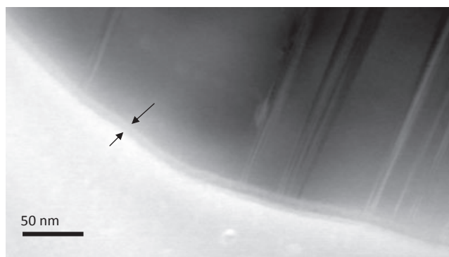
Fig. 8. TEM bright-field image of an irradiated rim (indicated by arrows) in Kapoeta.
