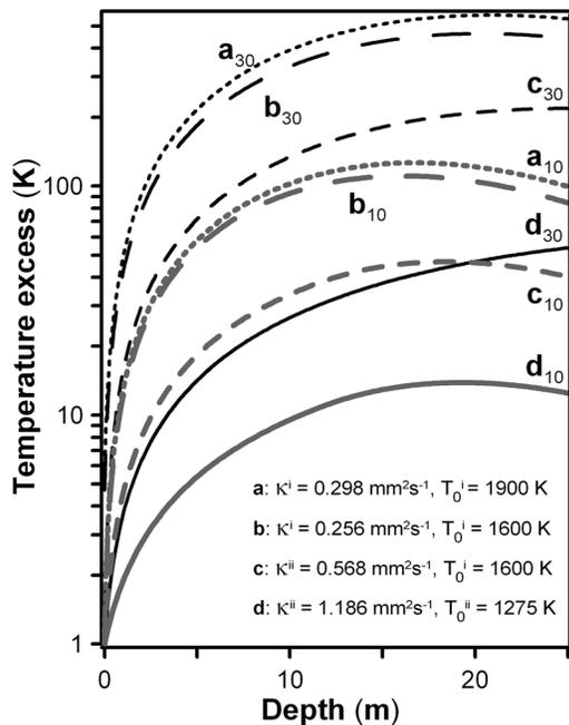
**Figure 1.** Temperature excess over near-surface atmosphere versus depth for a 15 year old lava flow having ultramafic (a), mafic (b, c), and felsic (d) composition. Subscripts denote flow thicknesses of 10 m and 30 m; superscripts indicate values from (i) *Davies et al.* [2005] and (ii) *Petovic and Dufek* [2005].
