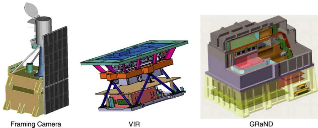
Fig. 5. Dawn payload, consisting of a framing camera, visible and infrared mapping spectrometer and gamma ray and neutron detector.
