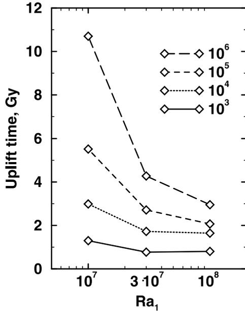
**Figure 3.** The dependence of the uplift time on the Rayleigh number for three-dimensional models with Arrhenius viscosity with  $\Delta\eta = 10^8$  and  $\exp(\theta) = 10^3, 10^4, 10^5$  and  $10^6$ .
